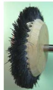
Angled view showing missing tufts and broken bristle
